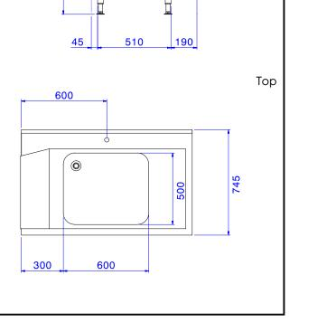
Handling System for Hood type Pre-wash Table with 600x500 Bowl Right to Left, 1200mm
